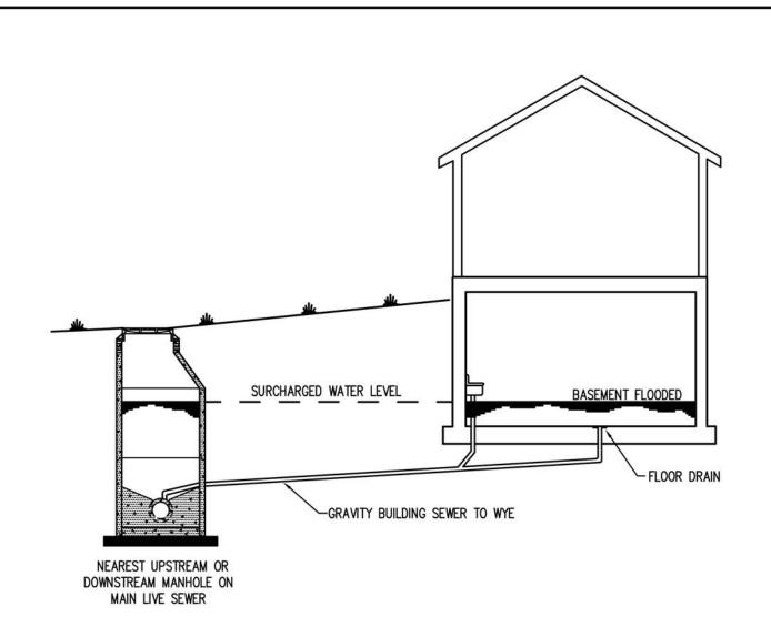
A SANITARY SEWER BUILDING CONNECTION CONSTRUCTED IN THIS SITUATION WILL NOT BE ACCEPTED
